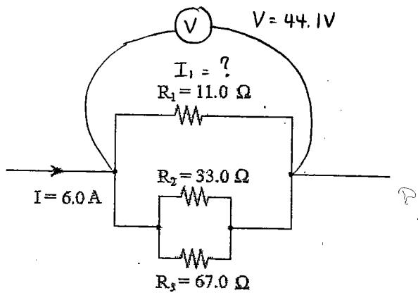
7. What is the voltage,  $V$ , of the power supply shown in the circuit?
