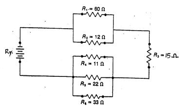
14. Solve the following circuits (find the current, voltage and resistance for reach element in the circuit).
