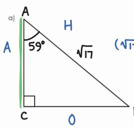
$$\angle B = 180^{\circ} - 90^{\circ} - 59^{\circ} = 31^{\circ}$$
